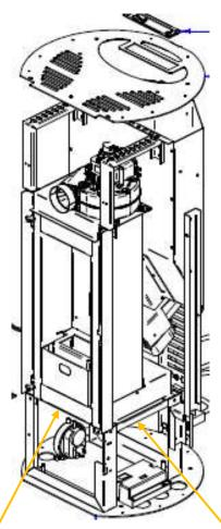
FOR THE CLEANING OF THE STOVE'S FURNACE IN THE FIRST SERIES, THE BOTTOM OF THE STOVE (WHERE THE FUME EXTRACTOR ENGINE IS FIXED) MUST BE DISASSEMBLED BY UNSCREWING THE VARIOUS SCREWS THAT ARE FIXING IT.
