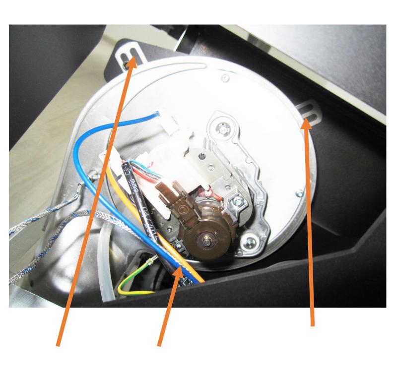
UNSCREW THE 3 SCREWS WHICH FIX THE
