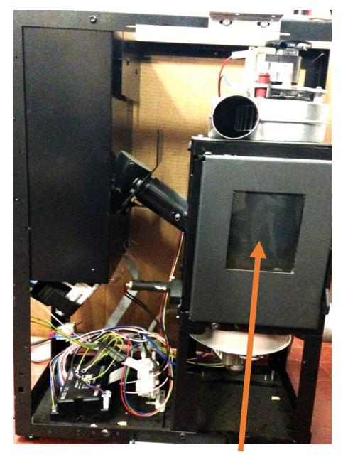
ASPIRATE THE INTERIOR PART OF THE CHAMBER OF COMBUSTION
