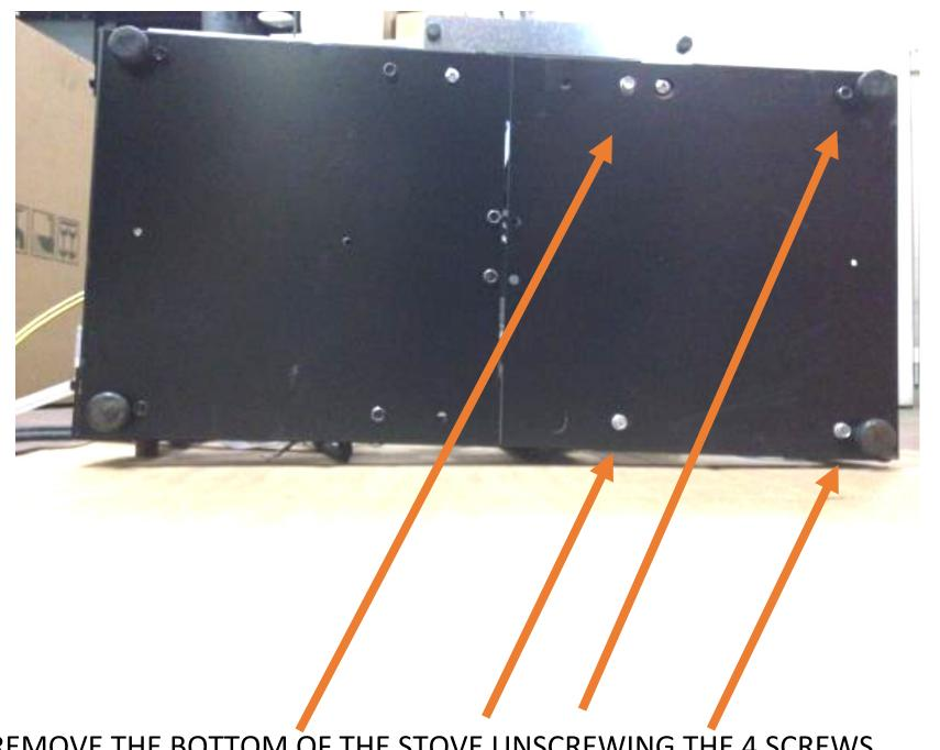
REMOVE THE BOTTOM OF THE STOVE UNSCREWING THE 4 SCREWS
