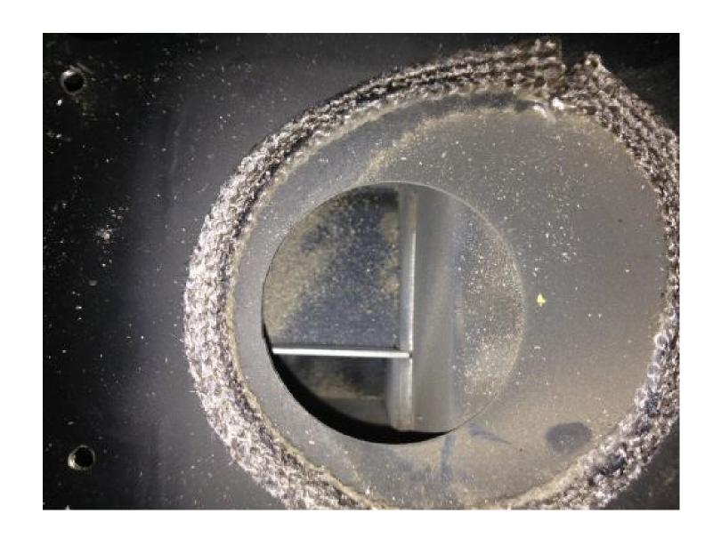
ASPIRATE THE FRONTAL PART OF THE SMOKE ROUTE, REMOVE THE FAN OF THE MOTOR FOR THE CLEANING AND CHANGE THE ADHESIVE ROPE
