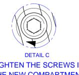
TIGHTEN THE SCREWS IN THE NEW COMPARTMENTS TO SUPPORT THE SMOKES MOTOR.
