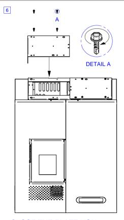
CLOSE THE PLATE YOU PREVIOUSLY REMOVED, TIGHTENING THE 4 SCREWS.
