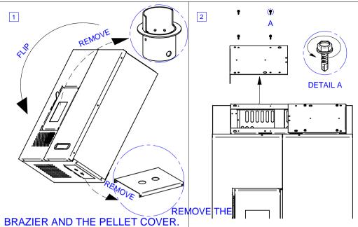
BRAZIER AND THE PELLET COVER. SUBSEQUENTLY, TURN THE STOVE UPSIDE DOWN LAYING THE TOP ON POLYSTYRENE OR CARDBOARD.
